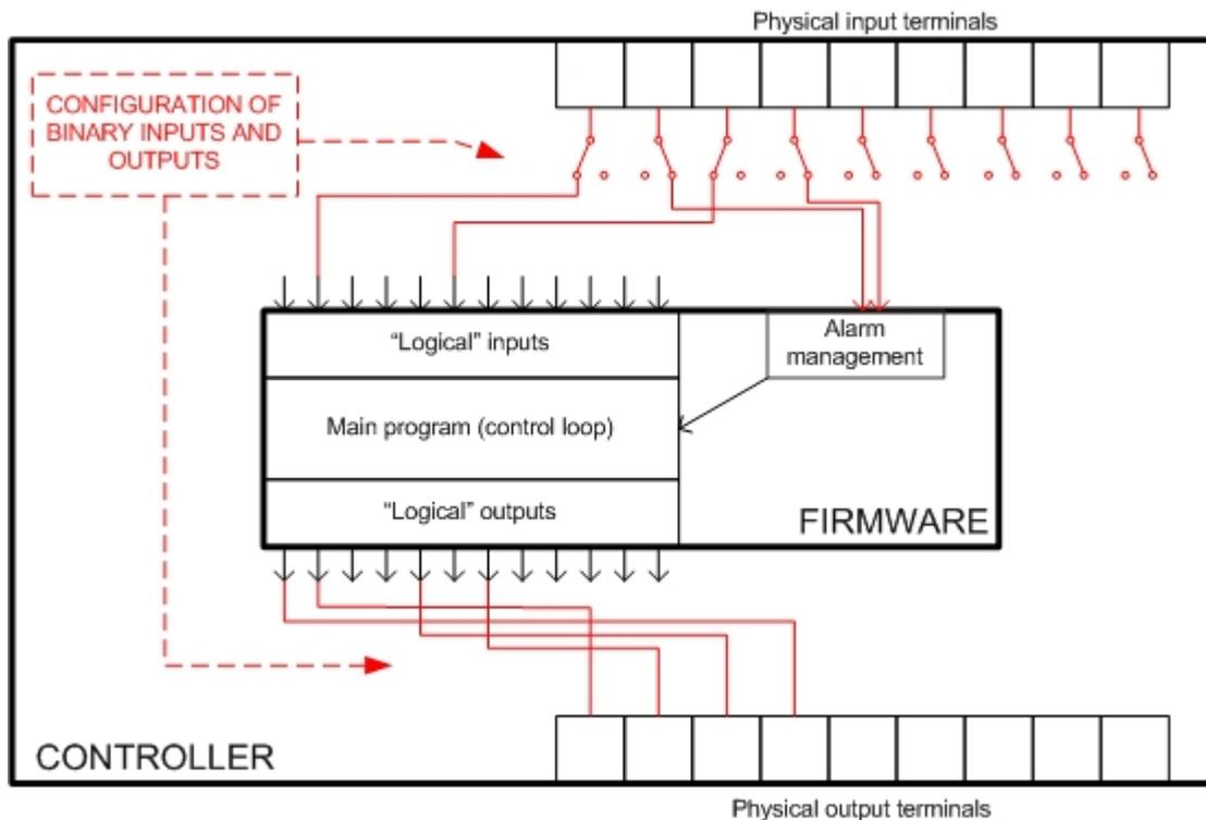
PRINCIPLE OF BINARY INPUTS AND OUTPUTS CONFIGURATION
