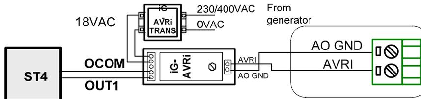
AVRi output is connected instead Remote voltage trimmer 470 ohm to terminals ST4. Module R726 is not required.
