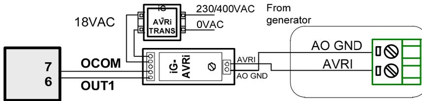
AVRi output is connected instead of external resistor for voltage adjusting.
