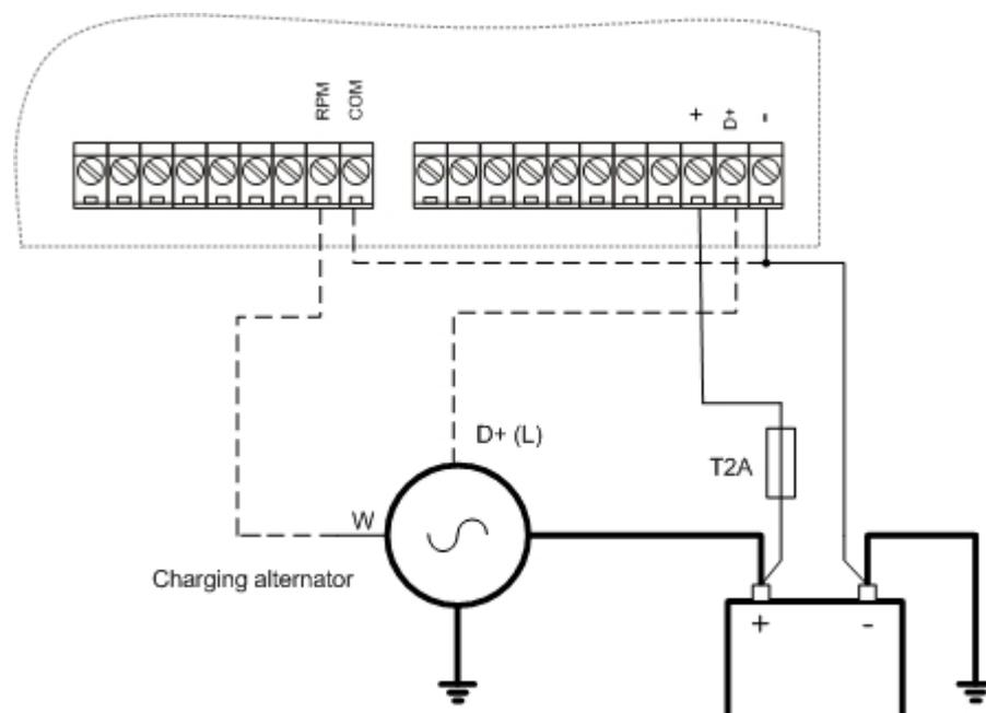
RPM is measured from generator frequency.
