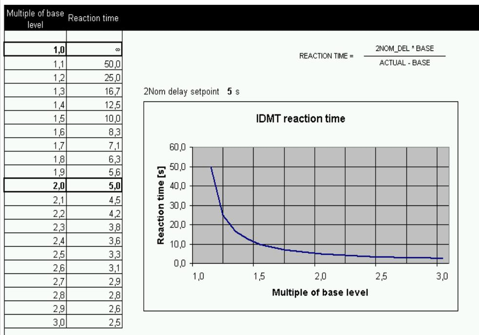
IDMT reaction time example (2Nom delay adjusted to 5s)
