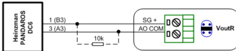
Terminals A3 and B3 are on OEM 14-pin connector.
