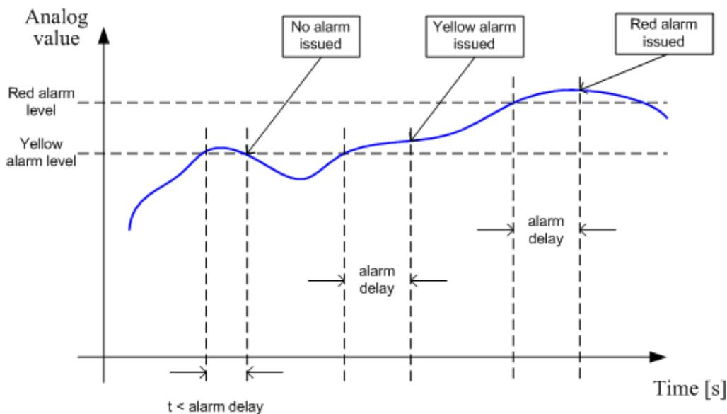
ANALOG INPUT ALARM EVALUATION PRINCIPLE
