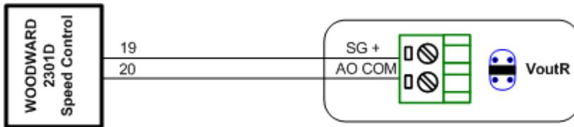
Terminals 19 and 20 are marked as analog inputs #1.
