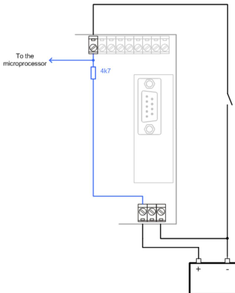
WIRING OF BINARY INPUTS
