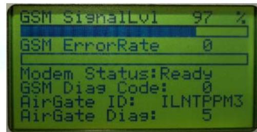
IL-NT GPRS MODULE AND GSM/GPRS SCREEN ON IC-NT DISPLAY
