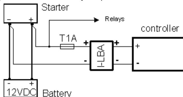
The I-LBA module ensures min. 350ms voltage dip under following conditions:
