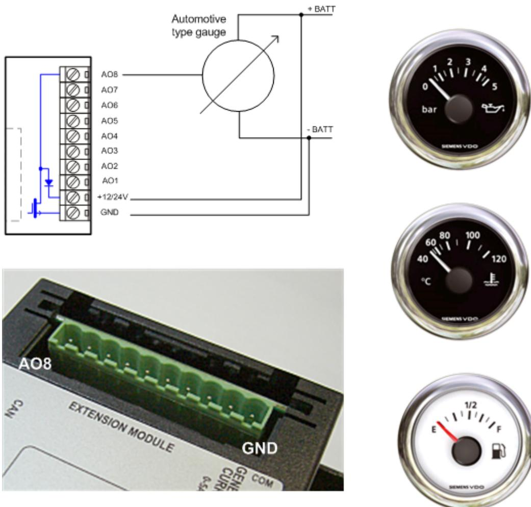
Examples of automotive gauges that can be used with the module:
