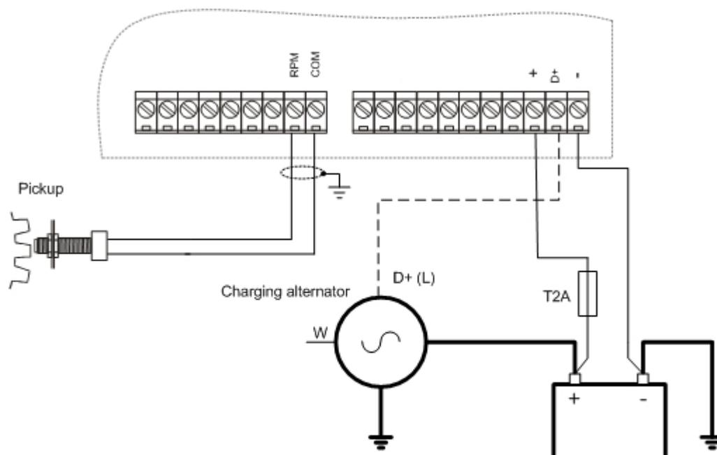
RPM measurement from the pickup.
