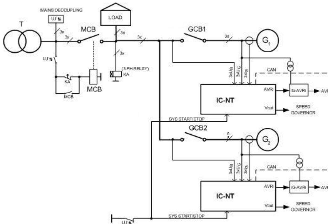
ISLAND-PARALLEL OPERATION WITH AMF AND WITHOUT PARALLELING
