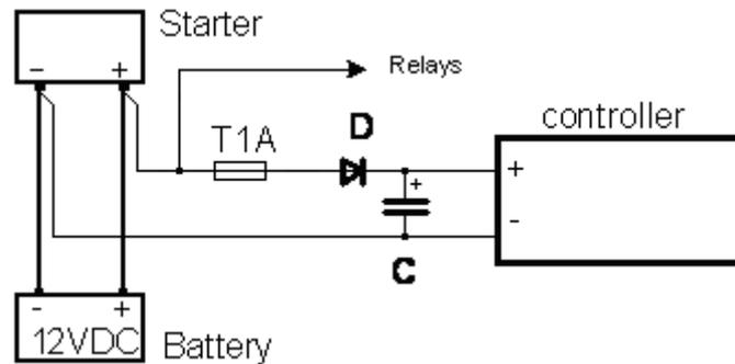
The capacitor size depends on required time. It shall be approximately thousands of microFarads. The capacitor size should be 5 000 microFarad to withstand 150ms voltage dip under following conditions:
