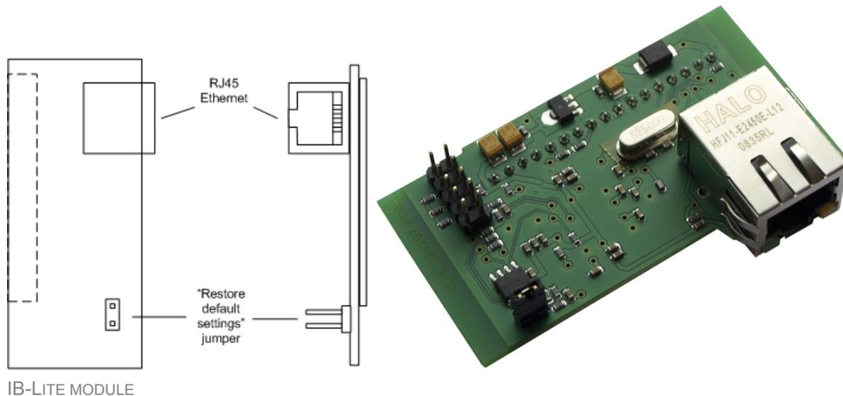
Use Ethernet UTP cable with RJ45 connector for connection of the module into your ethernet network. The module can be also connected directly to a PC using cross-wired UTP cable.
