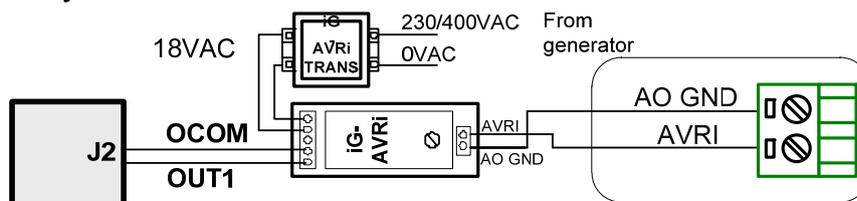
AVRi output is connected instead Remote voltage trimmer 470 ohm to terminal J2. Module R726 is not required.
