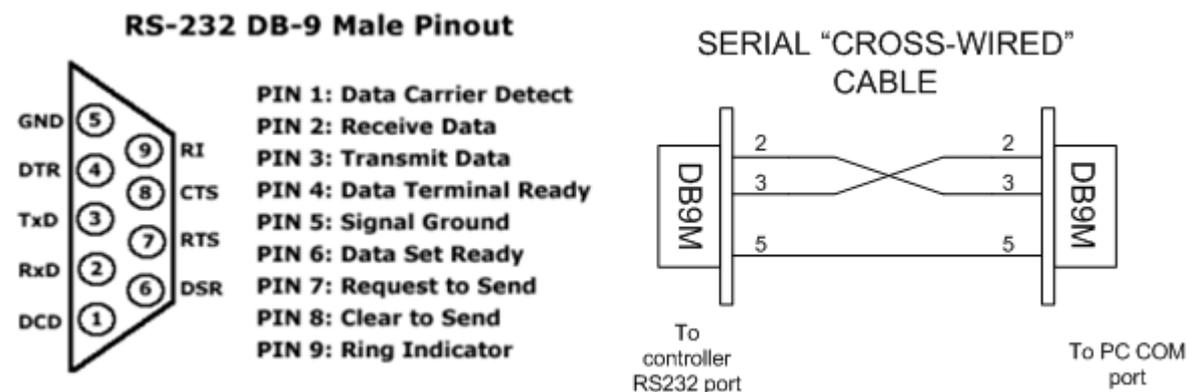
RS232 PINOUT AND CABLE WIRING
