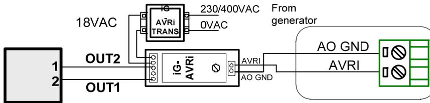
AVRi output is connected instead Remote voltage trimmer 100Kohm.
