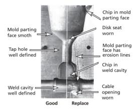
A CADWELD<sup>®</sup> mold is designed to last for an average of 50 connections. This will vary according to the care given the mold during use.
