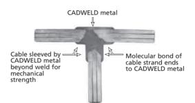
A CADWELD welded connection produces a joint (or connection) superior in performance to any known mechanical or pressure type surface-to-surface contact connector. By virtue of its molecular bond, a CADWELD welded connection will not loosen or increase in resistance over the lifetime of the installation.
