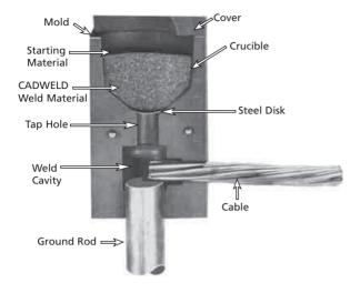
The CADWELD<sup>®</sup> process is a method of making electrical connections of copper to copper or copper to steel in which no outside source of heat or power is required.
